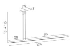
AXELL 120 is a suspension with a fixed reflector of 124cm, directed downwards
