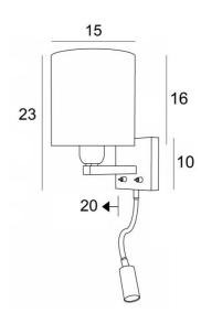
TEOS cyl is a wall light with a round cylindrical lampshade and reading light to be placed near a bed The arm has an E27 fitting with ring to fix the lampshade
