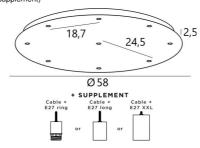
**CEILING BASE 9 o58** is a round ceiling base provided for nine outlets for hanging light bulbs, structures, glass or lampshades. In addition, standardised cabling is provided
