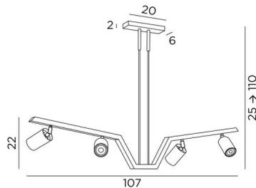
Elegant suspension. She reminds us of the flight of a beautiful bird in all its splendour ... Four movable spotlights are installed in all directions. They are equipped with GU10 bulbs, which work without a transformer. This luminaire is dimmable via an external dimmer. All bulbs are completely hidden inside the spotlights. **ALBATROS** is height adjustable and can easily be placed in a hallway or above a table
