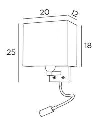
**TEOS rect** is a wall light with a rectangular lampshade and reading light to be placed near a bed The arm has an E27 fitting with ring to fix a lampshade
